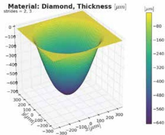
*Lens shape measured at 1-BM, APS.*
