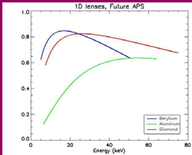
**CRL Normed flux availability for a 1D lens made in Be vs Al vs Diamond when focusing with  $p=46.7m$ ,  $q=56.5m$  and a lens number  $N$  between 1-95. By courtesy of Mati Meron APS, 2018.**
