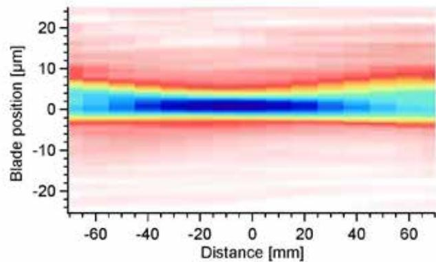
**Figure 2: Focusing capability of the GII lenses.**
