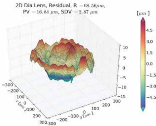
**Figure 1: Residual height error of a SCD lens. The doughnut like height error is systematic for the GII lenses.**
